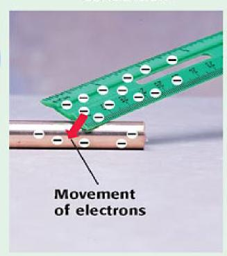
When a negatively charged plastic ruler touches an uncharged metal rod, the electrons in the ruler travel to the rod. The rod becomes negatively charged by conduction.
