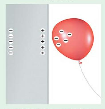
A negatively charged balloon makes a small section of a metal beam have a positive charge through induction. Electrons in the metal are repelled by and move away from the balloon.
